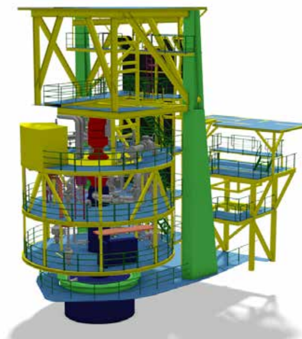
Fig. 4. 3D model of a scanned offshore platform.
